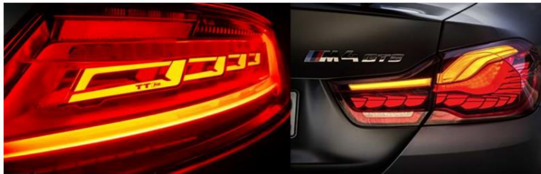
Figure 6.18 (a) Audi TT RS 2016 OLED Tail Light (b) BMW M4 Concept Iconic Lights OLED Tail Light
